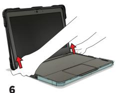
Push the left and right side clips down past the device, one side at a time, to release it from the bottom case.
