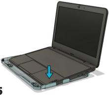
Slide the top case down, to secure the screen behind the side clips, until the device reaches
