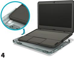
Carefully press the rear corner clips to snap onto the keyboard.
