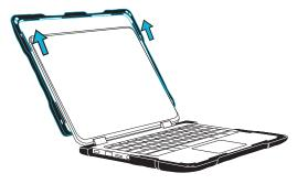
Gently push the rear clips down to unhook from the device.
