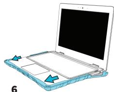
Press the lower side clips over the device, with pressure from both sides, to snap into place securely.
