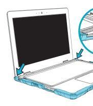
Start sliding the top case off by pushing up with your fingers on the bottom corners.
