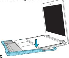
Slide the top case down, to secure the screen behind the side clips, until the device reaches the case's top edge.
