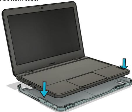
**The bottom shell is recyclable if the feet and foam are removed!**
