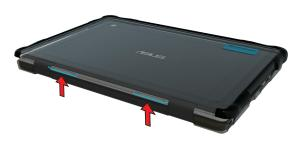
Start sliding the top case off by pushing up with your fingers on the bottom corners.
