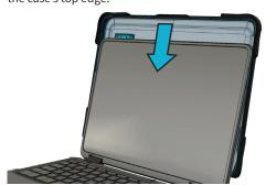
Carefully press the rear corner clips to snap onto the keyboard.
