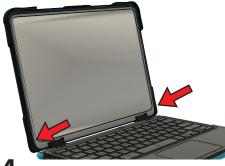
Push the left and right side clips down past the device, one side at a time, to release it from the bottom case.
