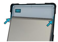
Push the keyboard forward until it is flush with the front edge of the bottom case.
