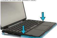
Start sliding the top case off by pushing up with your fingers on the bottom corners.
