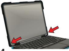
Push the upper left and right side clips outward to remove the top case from the device.
