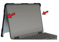
Gently push the rear clips down to unhook from the device.
