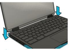
Push the left and right side clips down past the device, one side at a time, to release it from the bottom case.
